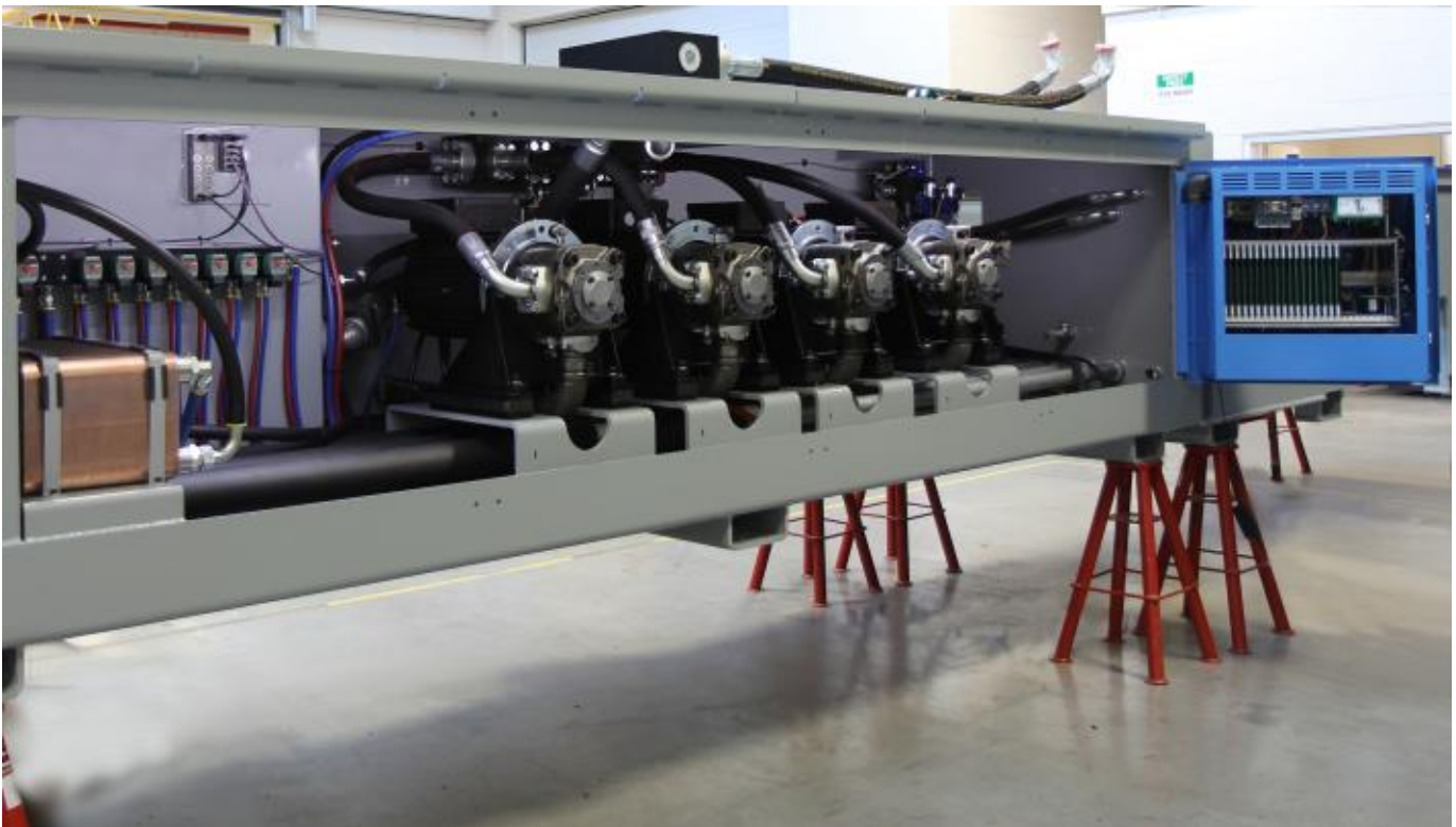
Easily accessible pump cabinet components. Photo taken during machine assembly.
