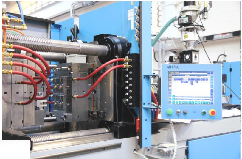
A150 closure system (above); molded parts (left)
