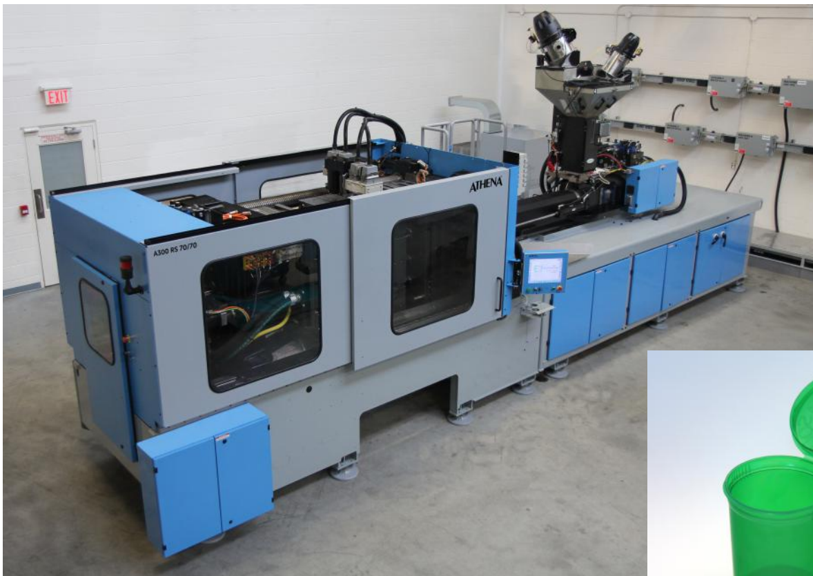
A300 stack mold carrier machine (above); 30-dram flip-top vial (right)
